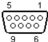
– View of sockets on the plug side or of sockets on the solder side.
