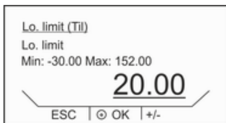
Fig. 32: Setting the temperature limit
