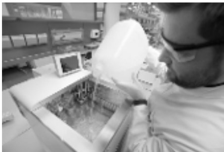
Fig. 24: Filling the bath thermostat
