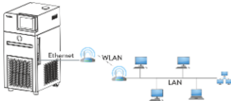
Fig. 16: Connected via LAN and WLAN
