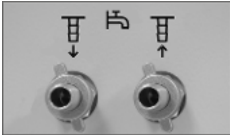
Fig. 72: Counter nuts on the cooling water nozzles
