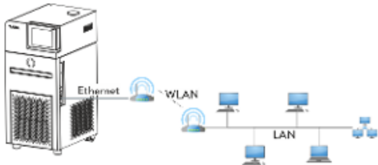
Fig. 16: Connected via LAN and WLAN
